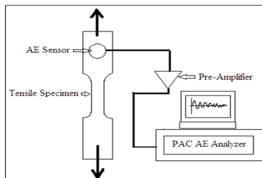
**Figure 1: AE Data Acquisition Setup**
