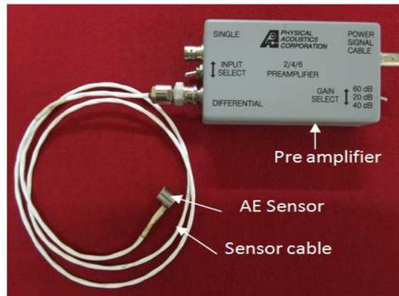
**Figure 2: PAC AE Sensor with Pre-amplifier**
