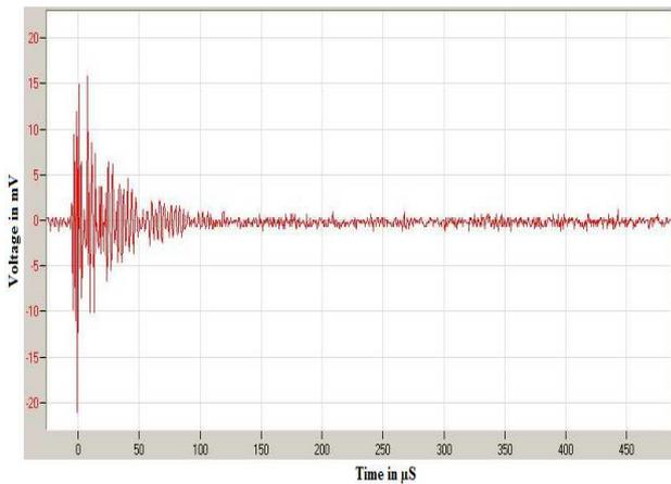
Figure 7: GFRP AE Waveform before Aging
