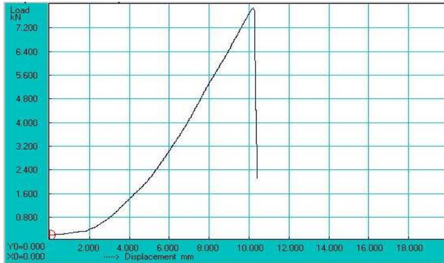
**Figure 3: Load Vs Displacement Curve (Without Aging)**
